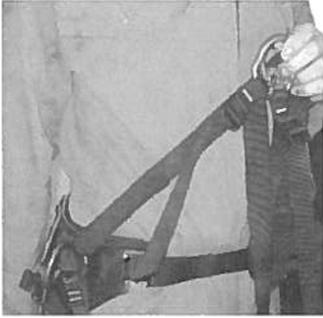
Pass the webbing of the two Legs of the Lower Part under the top of each of the two Lying Rings on the treeMOTION
