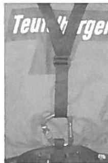
Connect the Accessory Karabiner to the Upper Rear Attachment Loop on treeMOTION harness
